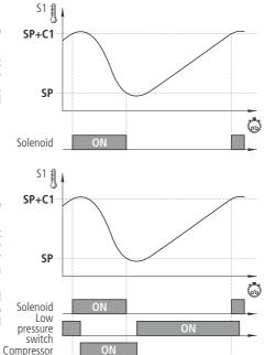
The compressor operates simultaneously with the solenoid valve, starting up when the latter opens and stopping when it closes.
