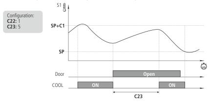
Management of door frame resistor (only devices with 5 relays)
