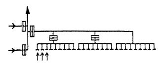
Figure 85 Now it is possible to adjust the airflow. The registers are combined in smaller groups, each with its adjusting damper.
