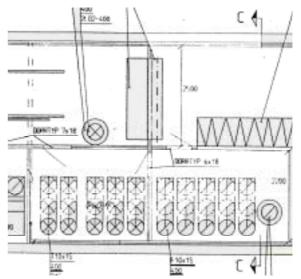
Figure 105 : Part of the fan room drawing with the extract air ducts to the right and the supply air ducts to the left. All these ducts are 400-mm diameter.
