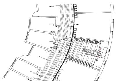
Figure 102 : The new supply and extract ducts are installed in the ceiling space and connected to the fan room and the different exercise rooms.
