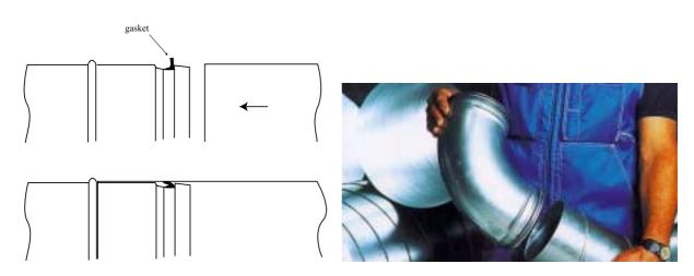
Figure 59. Pre-fitted sealing gaskets for circular ducts. Airtight rivets or plate-screws may be necessary to ensure the mechanical stability of the joint.
