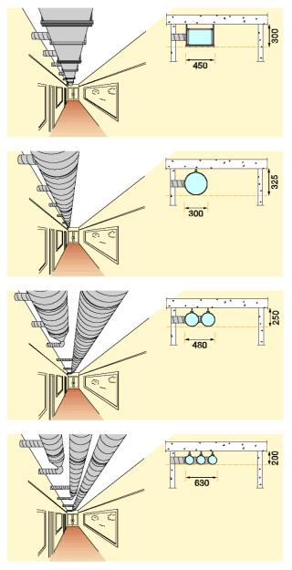
Figure 67 : Space demand for rectangular or circular duct(s)
