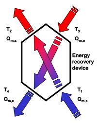
Figure 57. Schematic diagram of energy recovery principle. Subscript s and e denote the supply and extract sides, respectively.
