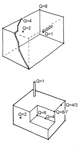
Figure 56 : The noise from a source will be influenced by the surrounding surfaces. The directivity factor Q equals 1 for full sphere and 8 for 1/8 sphere. Near the source each doubling of Q will result in a 3 dB noise level increase:  $\Delta L = 10 \cdot \log Q$ .
