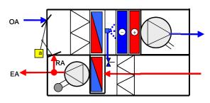
Figure 52 : To reduce the energy used for heating/cooling the AHU should either be equipped with a heat exchanger or – if the extract air has an acceptable quality – use return air. The shown unit has both possibilities!
