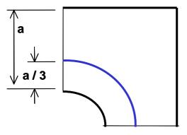
Figure 11 : Schematic representation of turning vane
