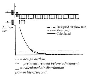
Figure 84 : Example on calculated and actual airflow distribution on a branch duct with 26 connected extract air registers. Each register comprises an adjustment damper. This example is showing a real installation before reconstruction!
