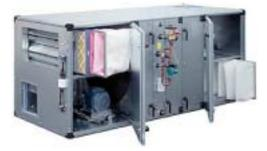
Figure 15 : Air handling unit for an SE system. The AHU includes two fans for the supply and extraction air streams and a heat recovery device including filters to avoid the fouling of the coils and the ductwork.
