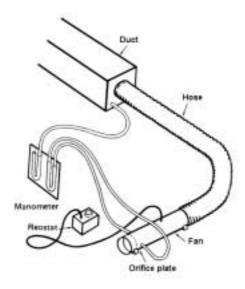
Figure 87 : Typical equipment used for tightness testing of ductwork.
