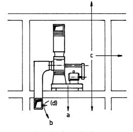
Figure 54 : The noise from the fan can spread in different ways and directions: Vibrations can result in structure borne noise (a) - Air borne noise carried through the ductwork (b) - Airborne noise in the fan room spreading to adjacent rooms (c), and noise emitted from other ductwork components such as dampers, registers etc (d).
