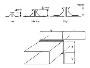
Figure 63 : Slip joints on rectangular ducts add to the space requirement. At installation free space has to be available for the joint connection.
