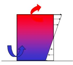
Figure 22 : The airflow differs between winter and summer due to the stack effect
