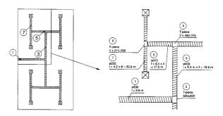
Figure 83 : Symmetrical ductwork where the supply air (entering at 1) passes through identical duct components on its way to the registers.
