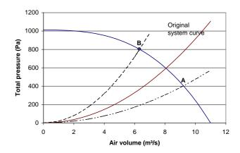
Figure 49 : Illustration of working points for fans
