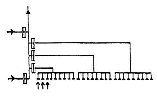
Figure 86 The same system once more solved with an alternative location of the adjusting dampers.
