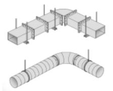
Figure 69: Hangers and joints for rectangular and circular ducts
