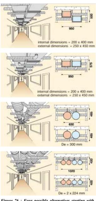
Figure 76 : Four possible alternatives starting with rectangular ducts followed by circular ducts.
