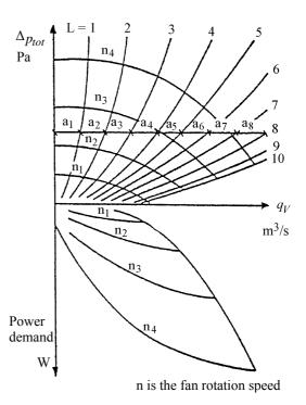
Figure 47: Fan graph with curves for different rotation speeds n, working lines 1-10, and power demand.
