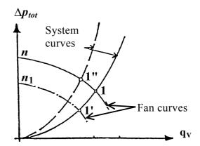
Figure 48: Illustration of the fan working point
