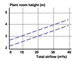
Figure 34 : Estimated room height for air handling installations
