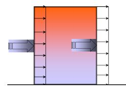
Figure 21 : Wind force on the façades affects the ventilation
