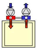
Figure 3. Schematic representation of balanced SE system. The air is mechanically supplied and extracted through two separate ducted systems. The air handling unit includes a heat recovery unit to transfer the energy of the outgoing air stream to the incoming air stream.
